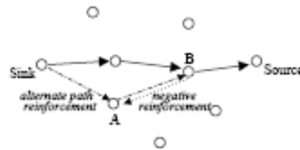
(c) Alternate-Path - Negative Reinforcement
